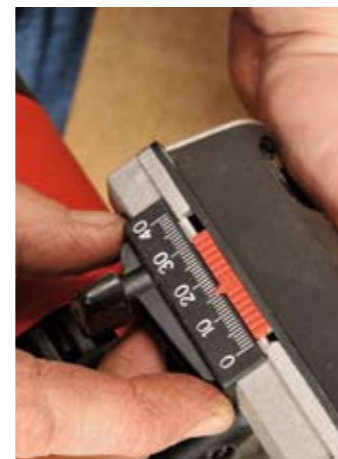
The dowel depth is set using the side scale; again it shows half the dowel length
