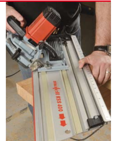
Performing a compound mitre cut: the F-clamps are not visible as they slip neatly into the underside of the track for extra security
