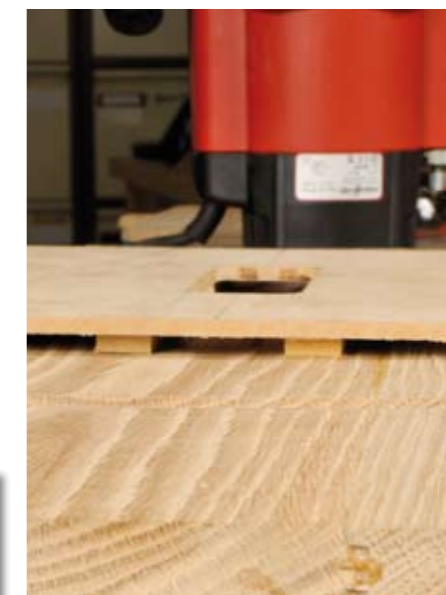
For template guide operations use thin MDF or ply. If it is thinner than the projection of the template guide stick some packers underneath with double-sided tape to get the right clearance
