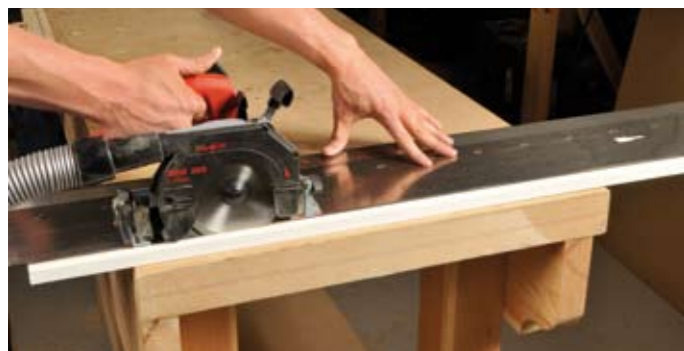
Using the 1.4m Flexi-Guide; it rolls up and clips together for storage in the case
