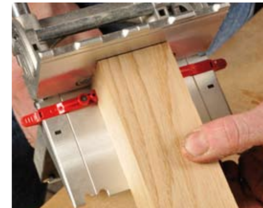
Use a pair of auxiliary stops for machining the ends of narrow components
