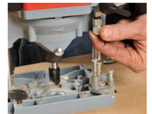
If the depth setting isn't quite right the LO65EC's fine adjuster makes minute changes incredibly easy to do
