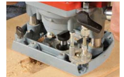
Machining a recess to take a sunk-in drawer pull
