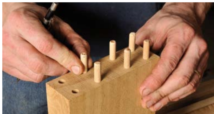
Pushing the dowels home
