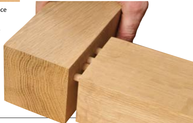
... and offset joints where one component is narrower than another, such as a table skirt, are also easy to achieve
