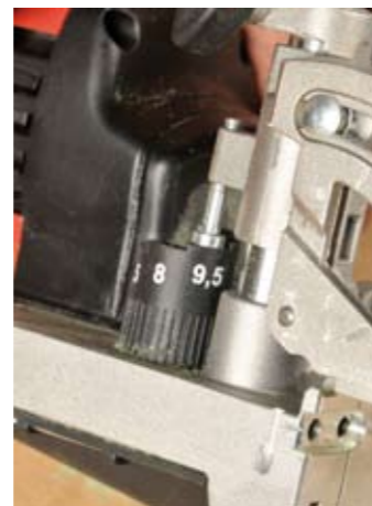
The material thickness is set using this turret; the measurement shown equal half the material thickness, thus 9.5mm equals 19mm stock
