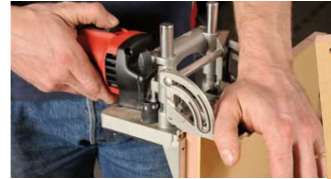
Face drilling using hand pressure to keep the fence located squarely on the workpiece. Safety note: take care to set the drill depth correctly just in case they come right through where your fingers are!
