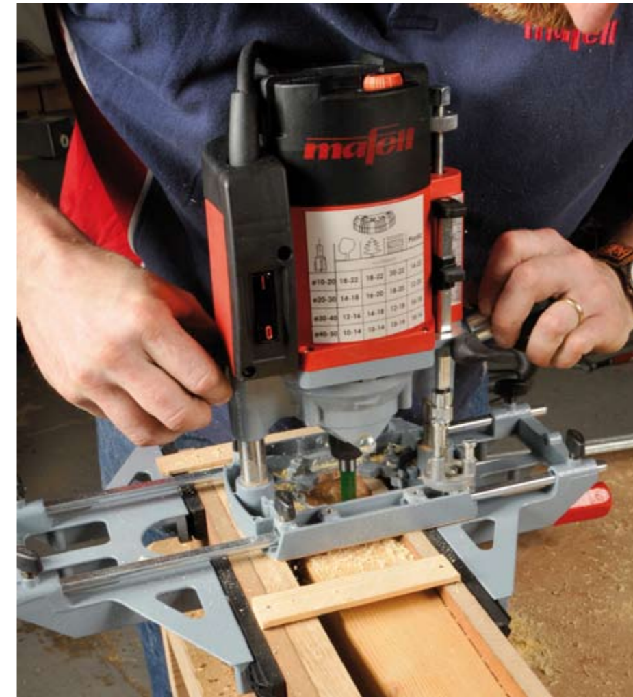
Machining a recess to take a sunk-in drawer pull
