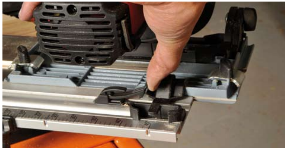
Lifting the clip that releases the saw from the guide rail
