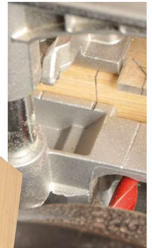
Lining up the detent with the pencil line ready to drill
