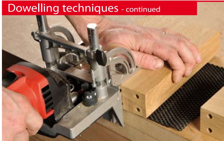
Making a trial joint in a rail to fit
