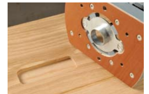
The finished recess very accurately machined thanks to the precisely engineered fit between the guide bush and the router base
