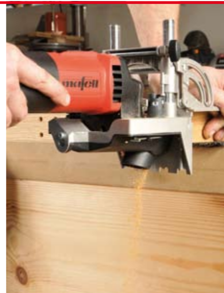
For picture clarity, we have not connected the extraction port to a vacuum unit. But note the machine drops its chippings conveniently in a stream rather than spraying them everywhere
