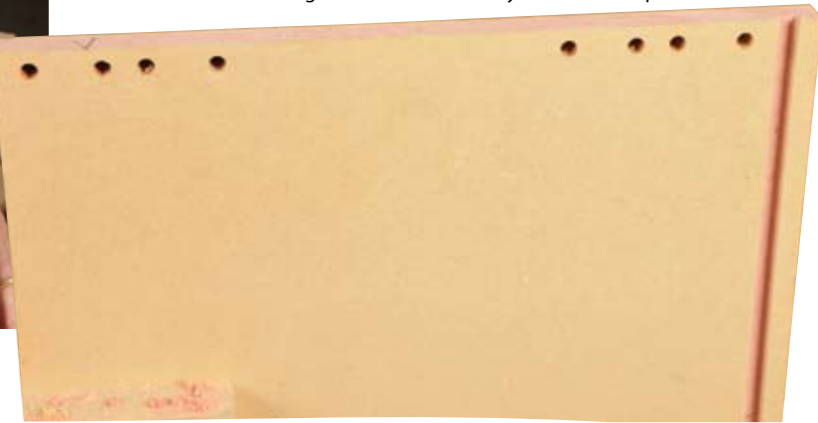
Two sets of 8mm drillings in a carcass rail ready to fit the side panel
