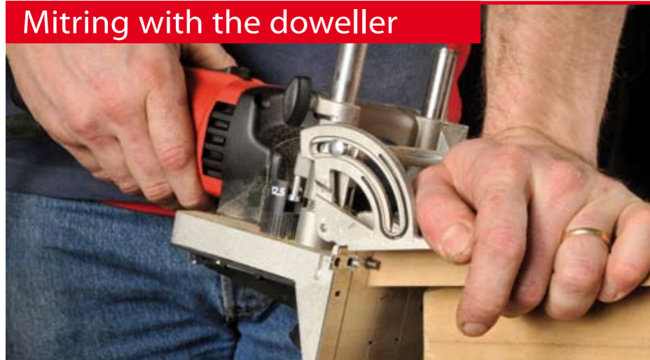
Dowel-drilling a 15° mitre by tilting the fence
