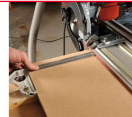
Setting the width for the next cut
