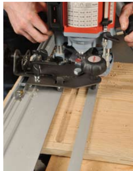
Machining a housing for a cupboard carcass. The fine adjustment makes it easy to increase the cut width
