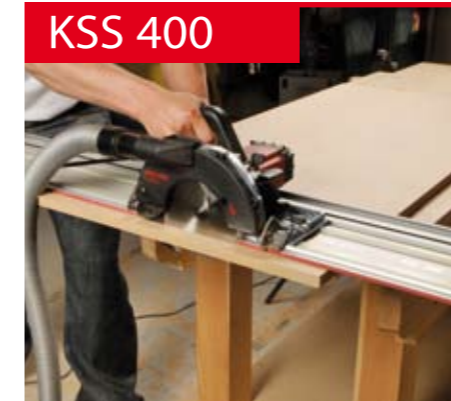
This trimming cut is being done without any clamping thanks to the rubberised grip surface underneath the guide rail
