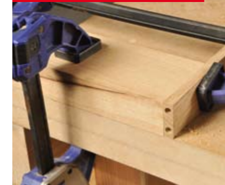
Even narrow window components can be dowelled together, note how it has been clamped to a larger block to facilitate machining
