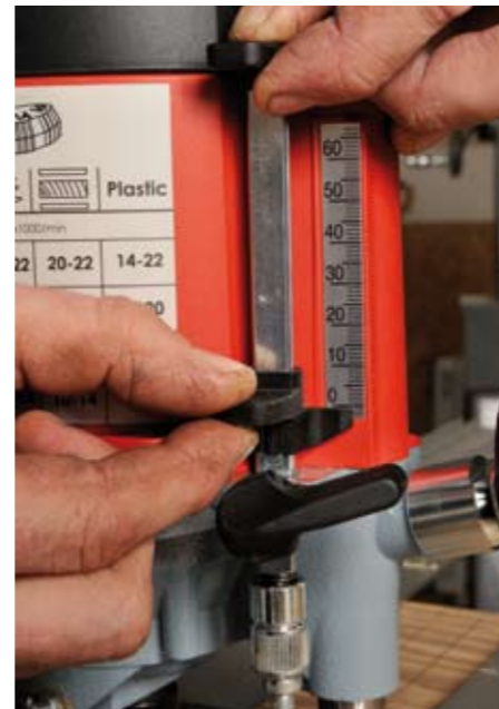
For very precise depth settings use a known object such as a drill shank to set the depth
