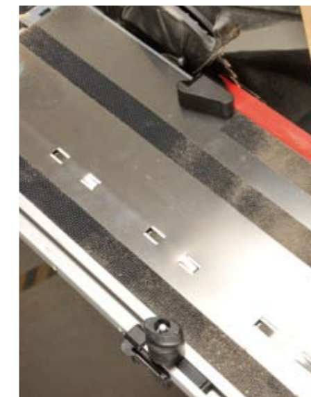
The underside of the guide rail showing the special pivot point and the adjustable angle guide
