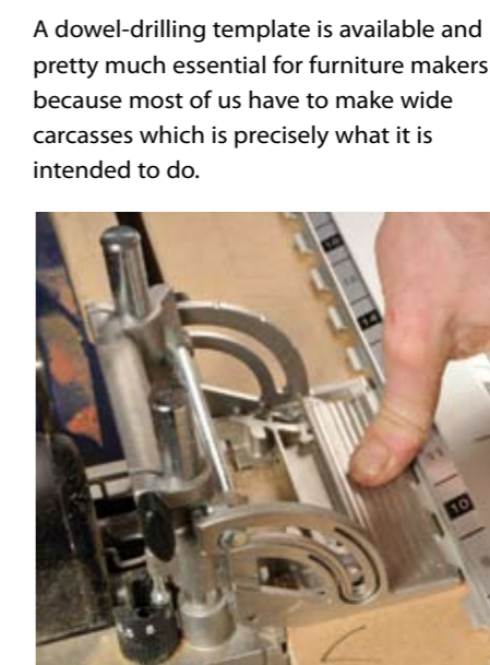
The technique for holding the Doweller against the jig
