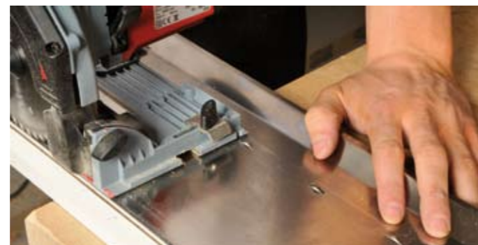
The saw is kept running true thanks to ingenious pressed guide pips
