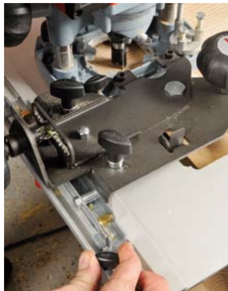
Setting the limit of the housing using the front lock knob. There is also a rear knob position
