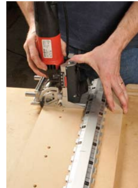
The 800mm Mafell dowel drilling template is intended for large panel work; note the pencil marks added on top to indicate which positions are actually going to be used
