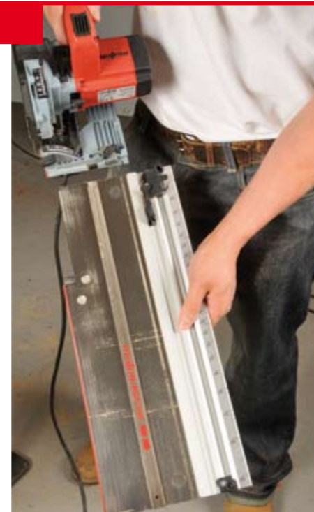
Simply pull the saw off the rail to detach it
