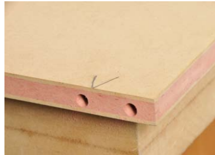
The resultant twin holes produced with 8mm cutters
