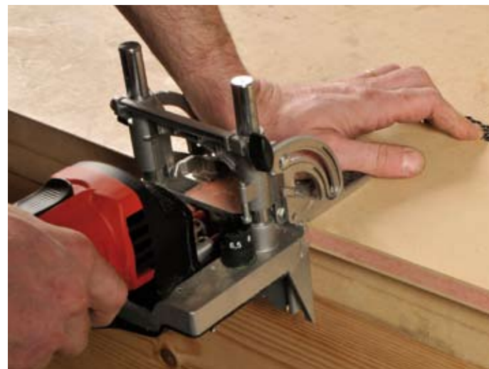
Machining the holes at the other end of the board to accept a narrow rail
