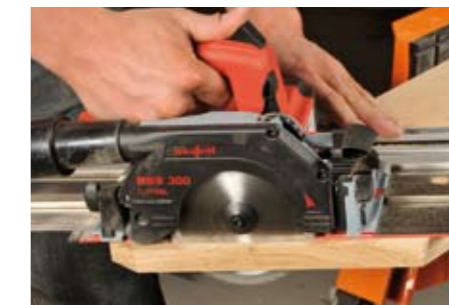
Making an angle cut: the scale can be reset time after time and still achieve accuracy
